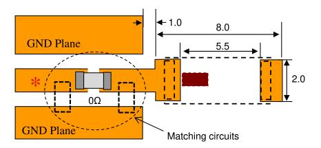
\* Line width should be designed to match 50ohm characteristic impedance, depending on your PCB material and thickness (distance to GND)
