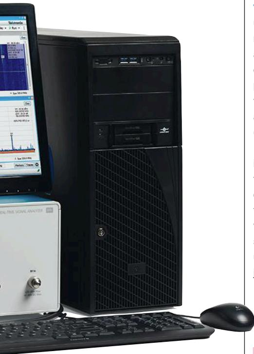
With IQFlow, the RSA7100A real-time spectrum analyzer can perform real-time digital-signal-processing algorithms and record/analyze long event sequences.
